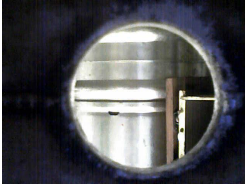
2(c) Internal Surface of Shive of Poor Cask: exposed aluminium
